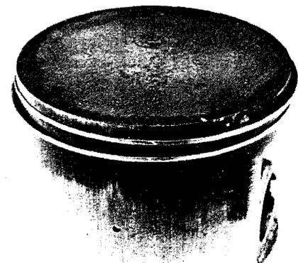
15:1 Adding oil reduced varnishing and raised the output 3.7 bhp over that obtained on 30:1 premix
